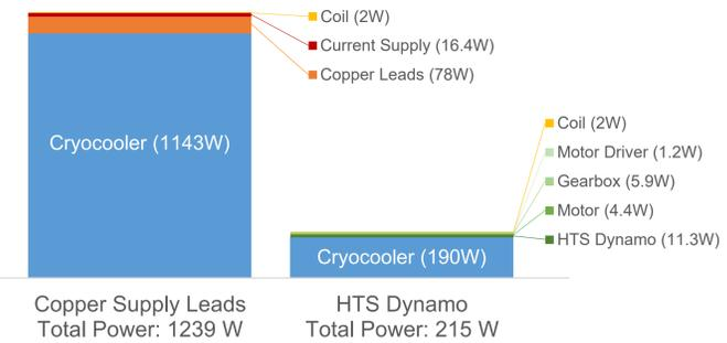
The total power, including cryocooler power, required to supply a 1000 A at 77 K with 2 W is significantly reduced when a HTS dynamo is used as the constant current supply.
