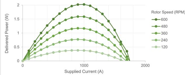
The varying magnetic field of the dynamo produces AC loss in the HTS. These losses produce heat in the cryogenic environment. The losses in a pair of 1 m long copper leads optimised for each supplied current, as calculated using the method from [2], are also plotted.
