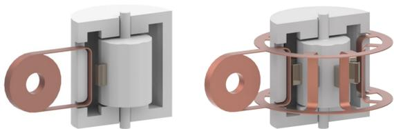
In this work, the efficiency of an eight stator, four magnet dynamo was measured by monitoring the shaft torque and dynamo DC output voltage across a range of rotational speeds and dynamo output currents.
