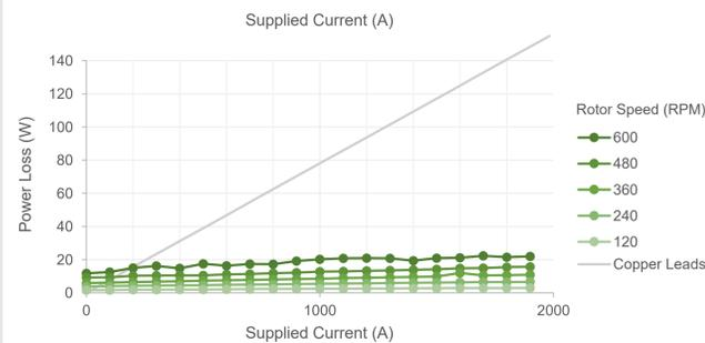
Across the speed range tested the efficiency of the HTS dynamo is between 10 and 16%. As shown in the above plot, the power required to provide 1000 A in the cryogenic environment is significantly less than is required using the standard method.
