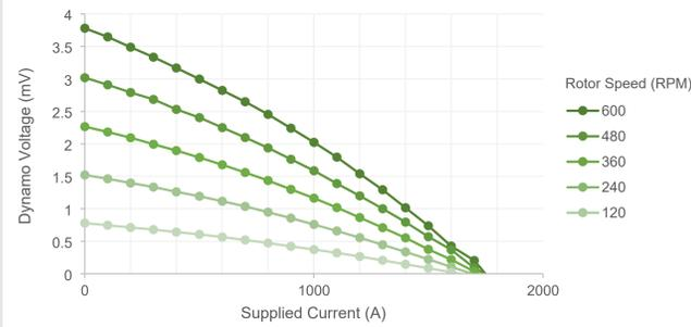
The output power of this HTS dynamo was found to be 2 W at the maximum speed tested. The optimum operating point in terms of power delivered to the HTS circuit occurs at 1000 A.
