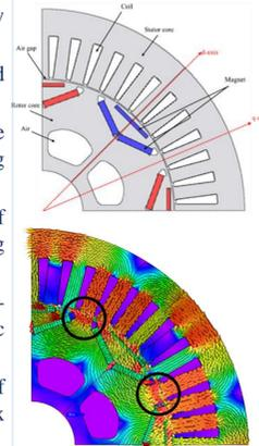
$$T = \frac{p}{2} \left\{ \varphi_f i_q + (L_q - L_d) i_q i_d \right\} \quad (\text{Equation of torque})$$
