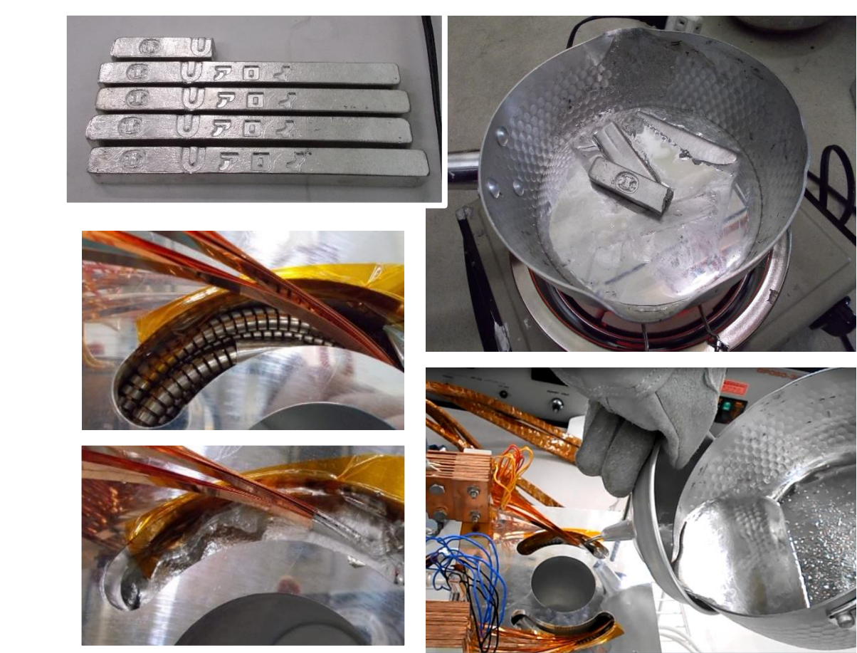
Fig. 2 Impregnation using low-melting point metal U-78 ( Sn-type alloy, produced by Asahi Metal Co., Ltd., m. p. \sim 78 \text{ }^\circ\text{C} )
