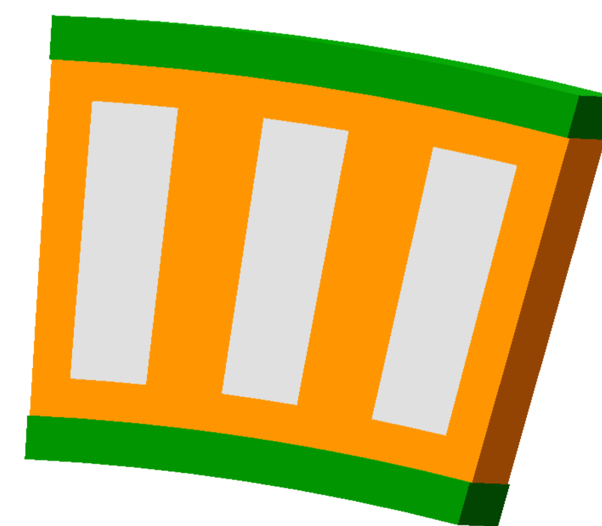
Fig.9. iron inserted into the armature winding
