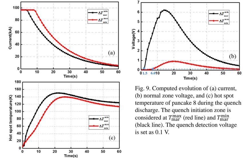
Fig. 9. Computed evolution of (a) current, (b) normal zone voltage, and (c) hot spot temperature of pancake 8 during the quench discharge. The quench initiation zone is considered at  $T_{mar}^{max}$  (red line) and  $T_{mar}^{min}$  (black line). The quench detection voltage is set as 0.1 V.
