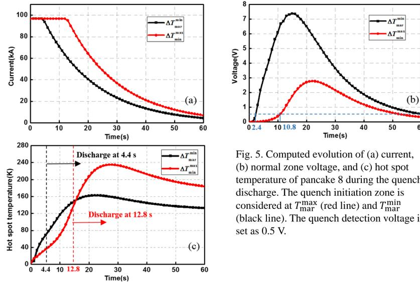
Fig. 5. Computed evolution of (a) current, (b) normal zone voltage, and (c) hot spot temperature of pancake 8 during the quench discharge. The quench initiation zone is considered at  $T_{mar}^{max}$  (red line) and  $T_{mar}^{min}$  (black line). The quench detection voltage is set as 0.5 V.
