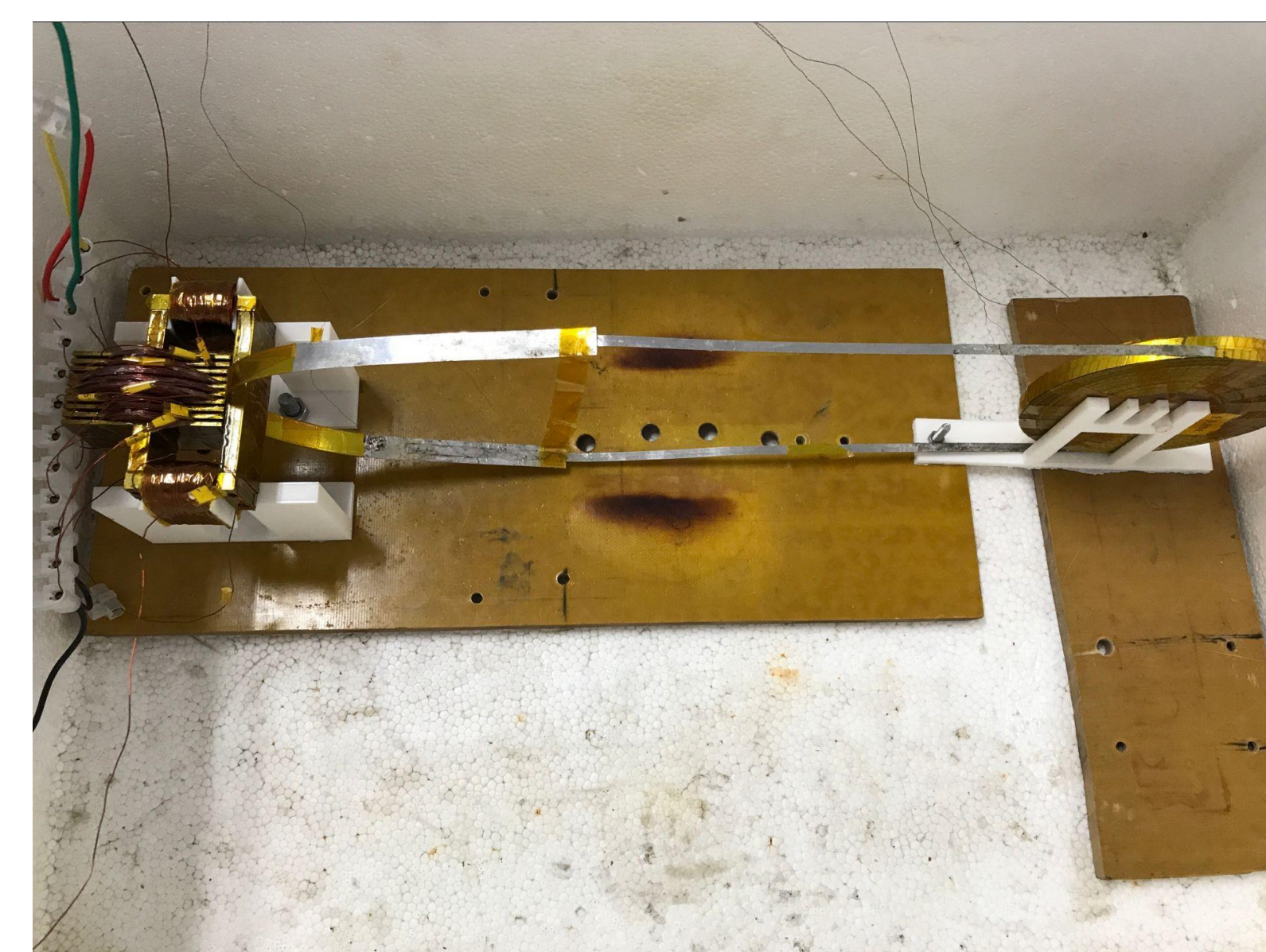
Fig. 2. The experimental setup of the newly mini-type HTS flux pump device.
