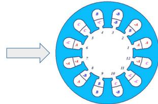
Table.2 Slot phase diagram of Spp=2/5 combinations for proposed FSCW
