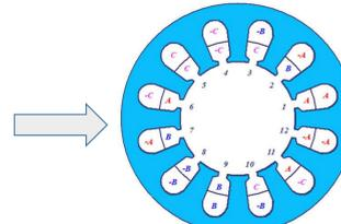
Two different FSCW topologies for 10-pole, 12-slot combination
