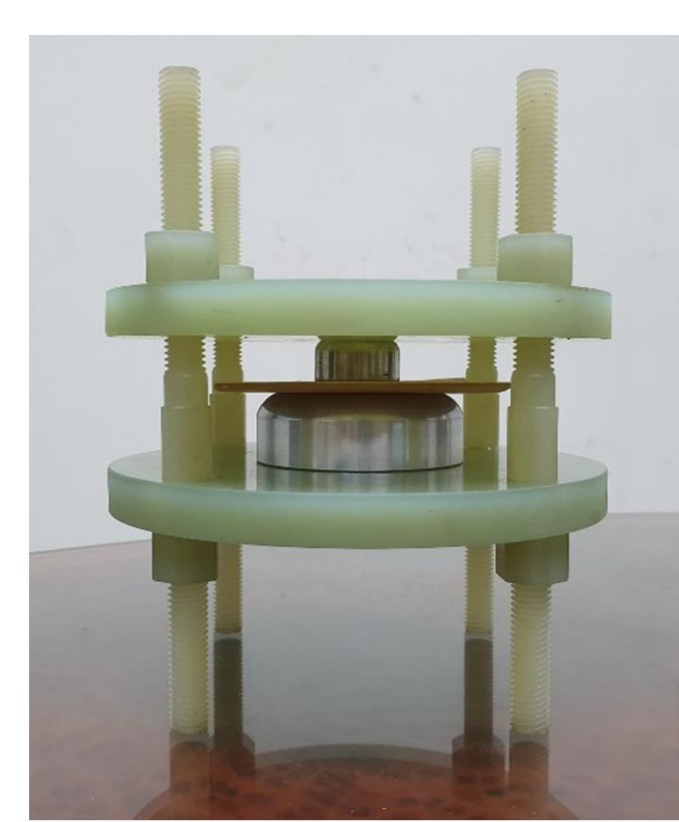
Fig. 1 Configuration of test jig and artificial defect
