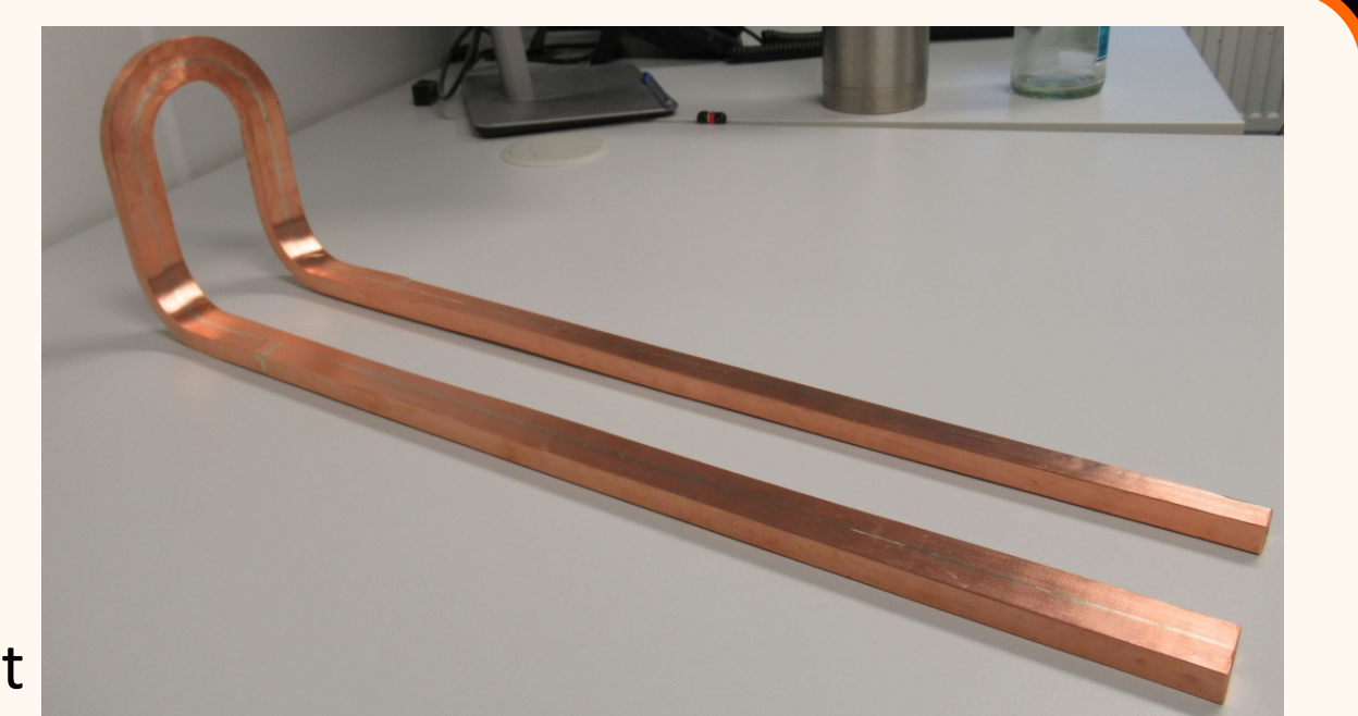
Test soldering of a piggyback conductor. Wedge shaped conductor in background.
