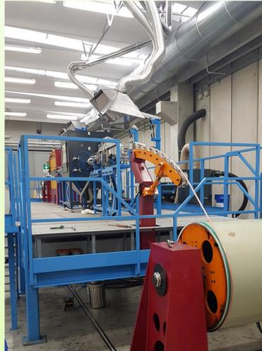
ICAS, set up a production line to process copper conductors to be used in magnets for fusion reactors, in order to prepare, apply and cure a cyanate ester based primer, aimed to improve the adhesion of epoxy resin insulation to copper.
