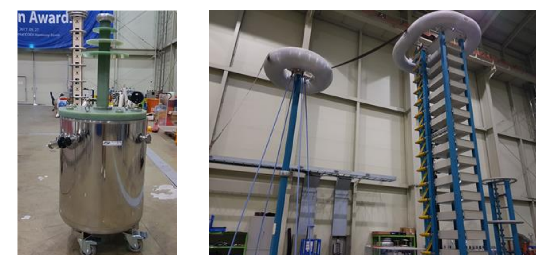
Test set up for the lightning impulse breakdown test
