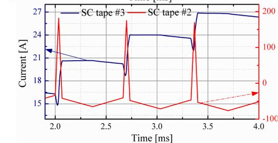
Fig. 5. Detailed waveform of bridge current  $I_2$  and load current  $I_3$  in three periods.
