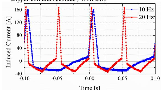
The induced current in the charge loop for different applied frequencies
