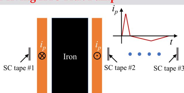
Fig. 3. Schematic of the 2D finite element model for self current driving HTS flux pump.
