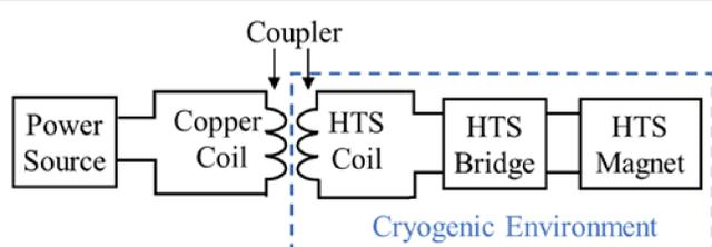
Fig. 1. Schematic structure diagram of the contactless rectifier type HTS flux pump.
