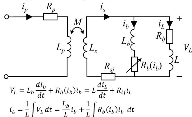
Fig. 2. Circuit model for the contactless rectifier type flux pump.
