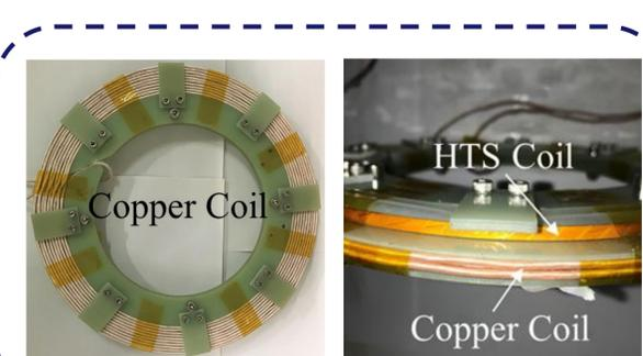
Fig. 7. The magnetic coupler is composed of a primary copper coil and secondary HTS coil.
