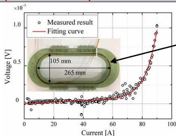
Fig. 6. Photo of the Load race-track coil.
