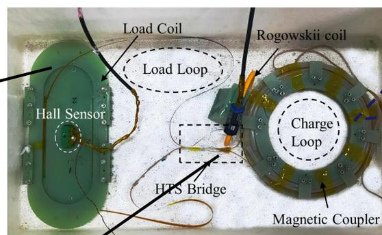
Fig. 8. Experimental scenario of the contactless self current driving HTS flux pump system
