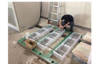
Fig.XIII Salt water dummy load for discharge test.
