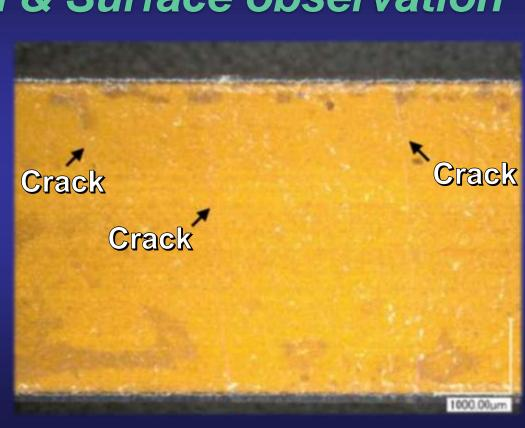
Several cracks are observed at the 1st trial with the target film thickness of 50 µm. There is no crack in the 2nd trial with the target film thickness of 30 - 10 µm and the heat treatment temperature of 100 °C.
