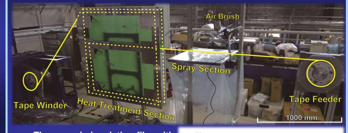
The ceramic insulating film with an average thickness of 19 µm is formed over an 8 m section of long REBCO tape. However, there is a large variation in film to application and tape winding. The quality control by automation is essential for tapes longer than several tens of meters to wind practical coils.
