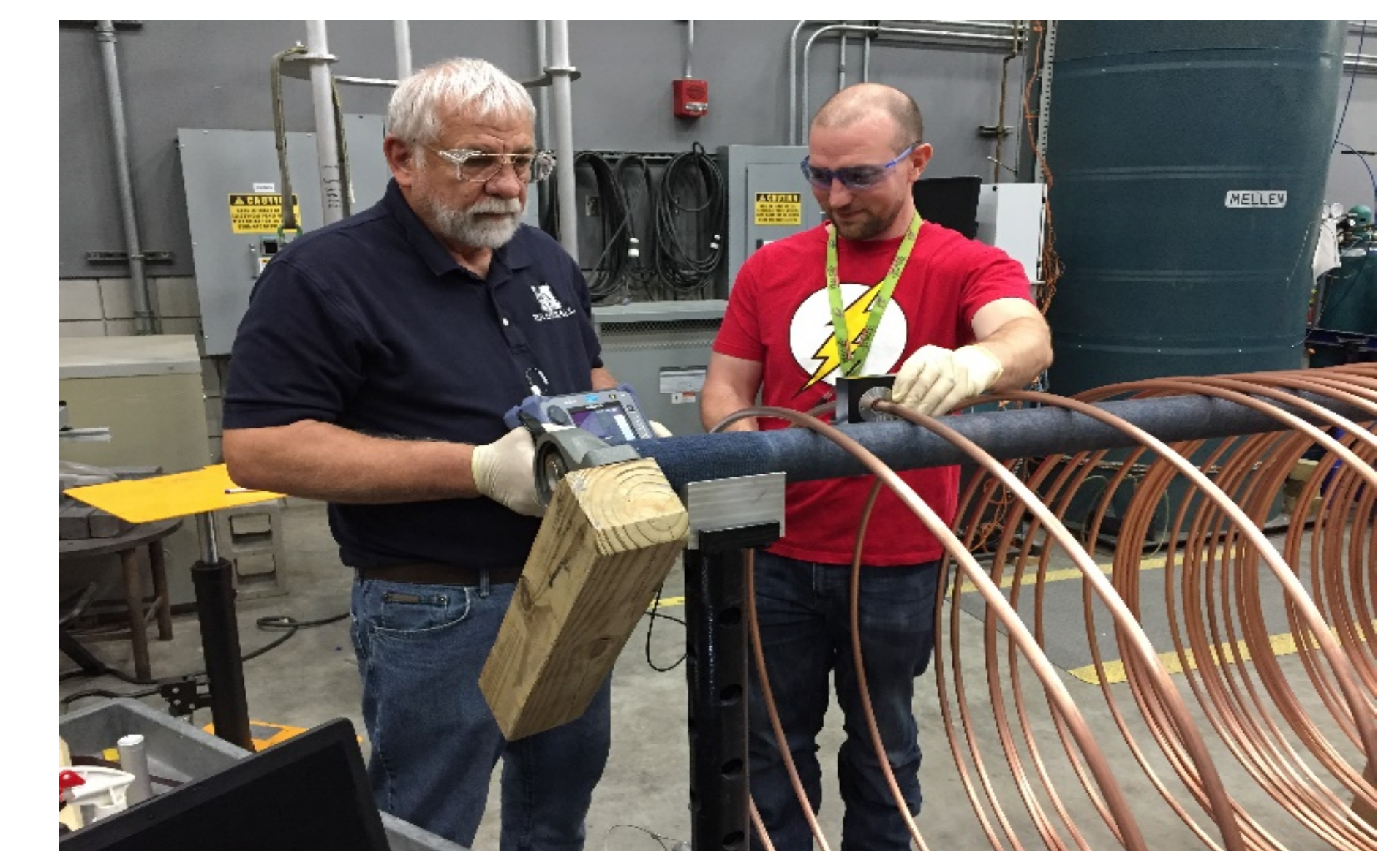
Long length eddy current testing capability for AL60 wires and precursors are developed. This picture shows surface inspection of 0.54" diameter long-length AL60 precursor wire has been developed.
