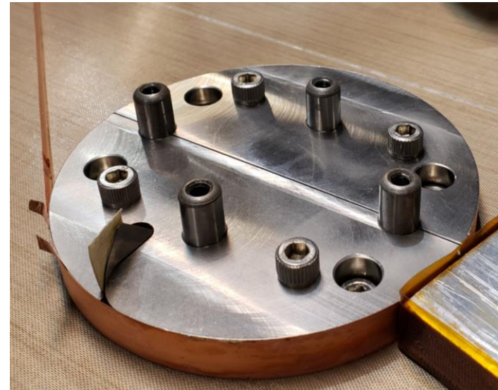
Above: Solder first turn to itself to secure inner part of coil for reusable bobbin removal
