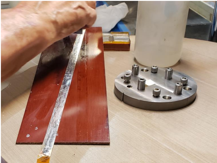
Above: Tin first turn for future leads and or coil inter-connections – HTS side FACING bobbin
