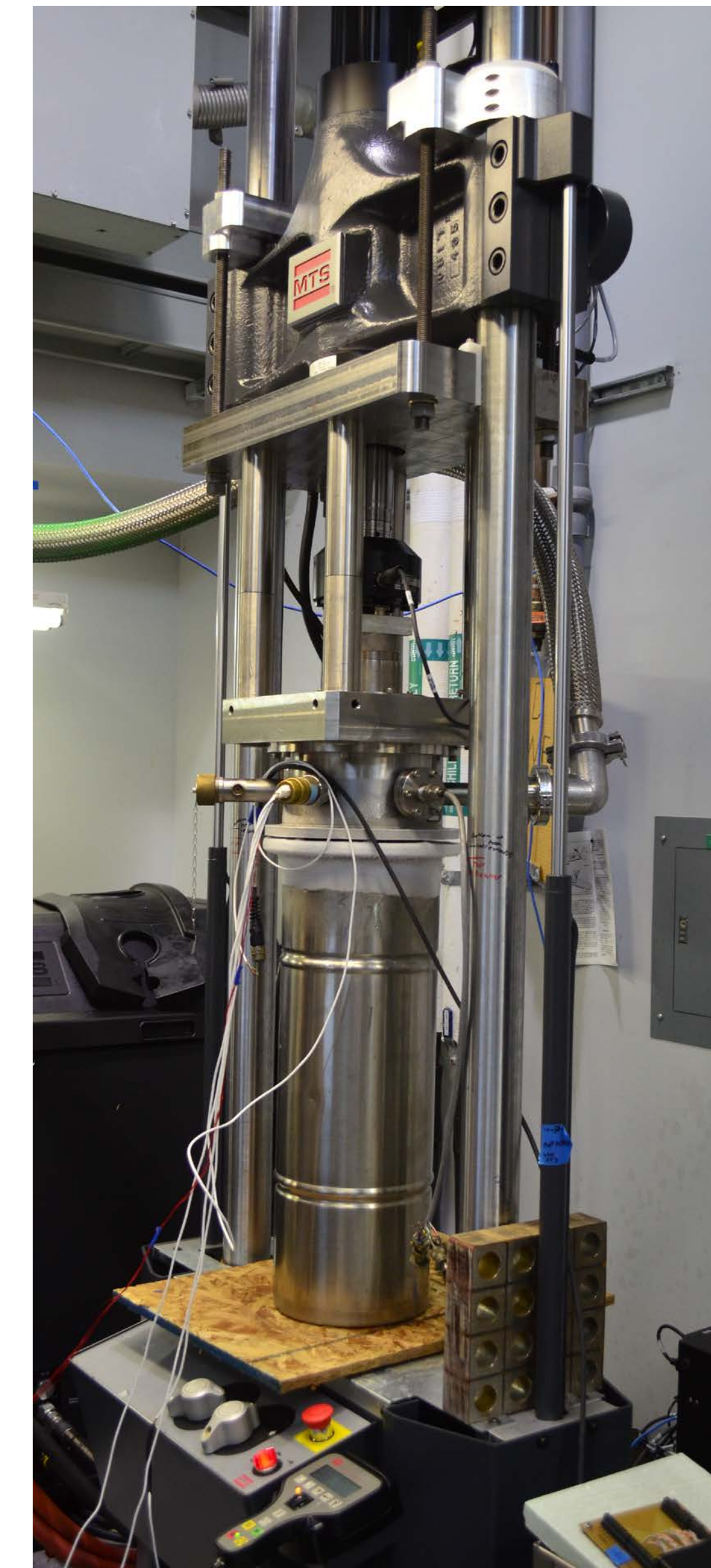
Mechanical test facility with cryostat in place and test in progress
