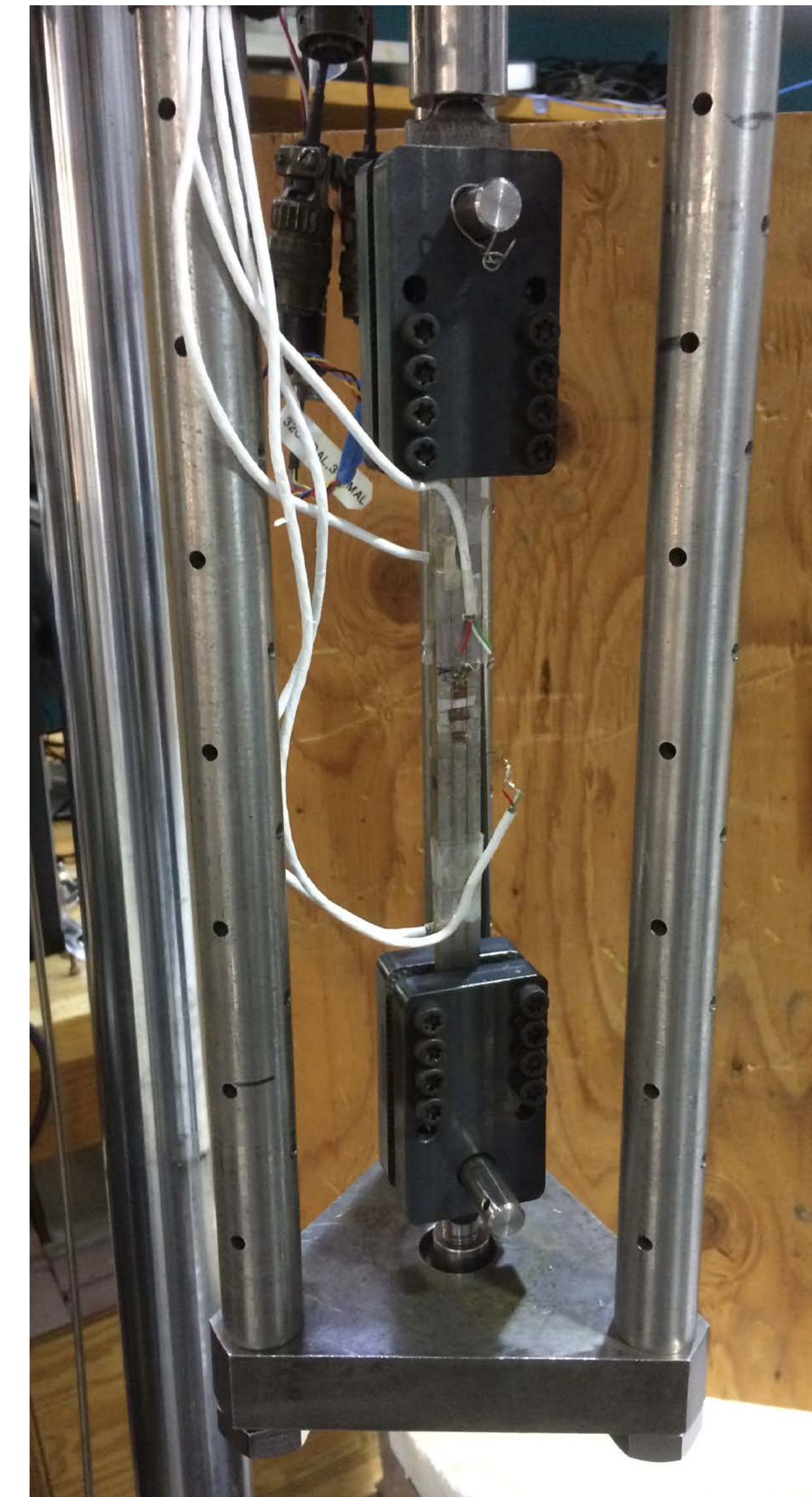
Re-entrant load frame with tensile specimen mounted in grips
