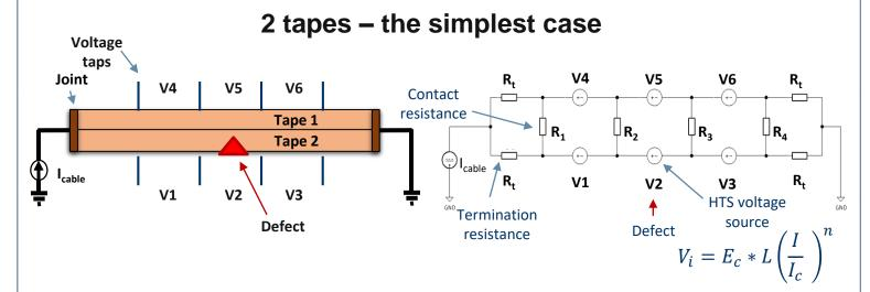
Model for Monte Carlo simulations to study the impact variations in  $I_c$  and n-value on the cable performance
