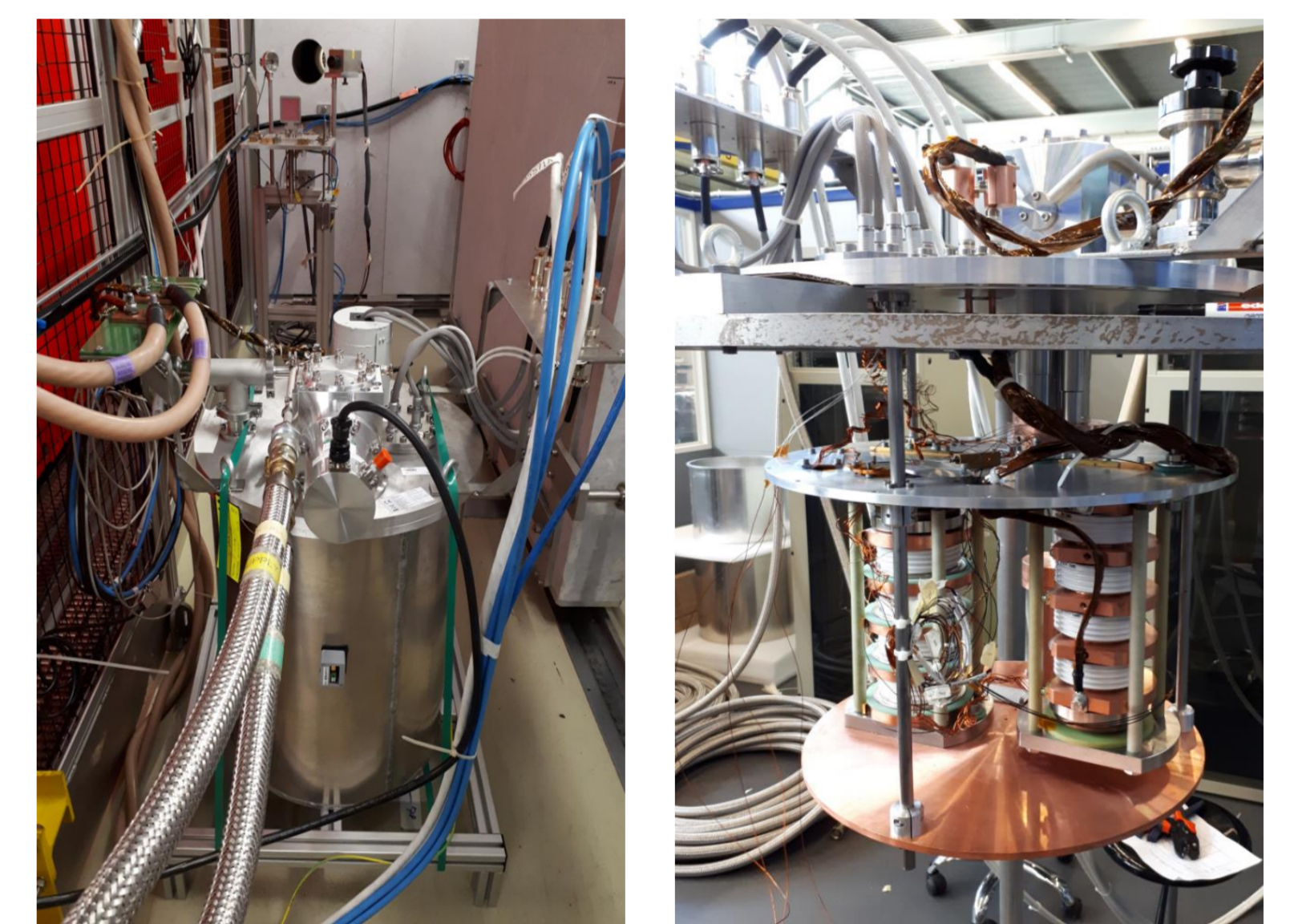
Cryostat containing diodes installed in the target area of CHARM
