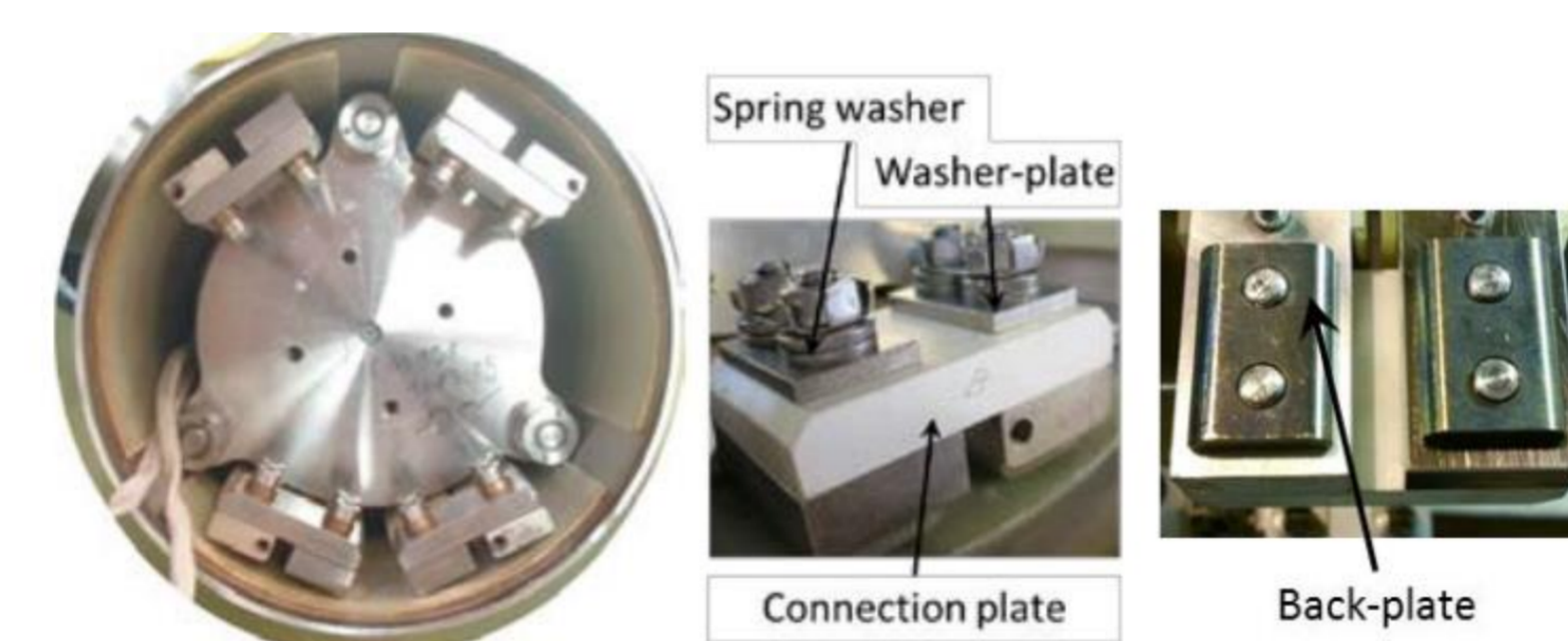
Quadrupole diode stack with bolted connection before consolidation
