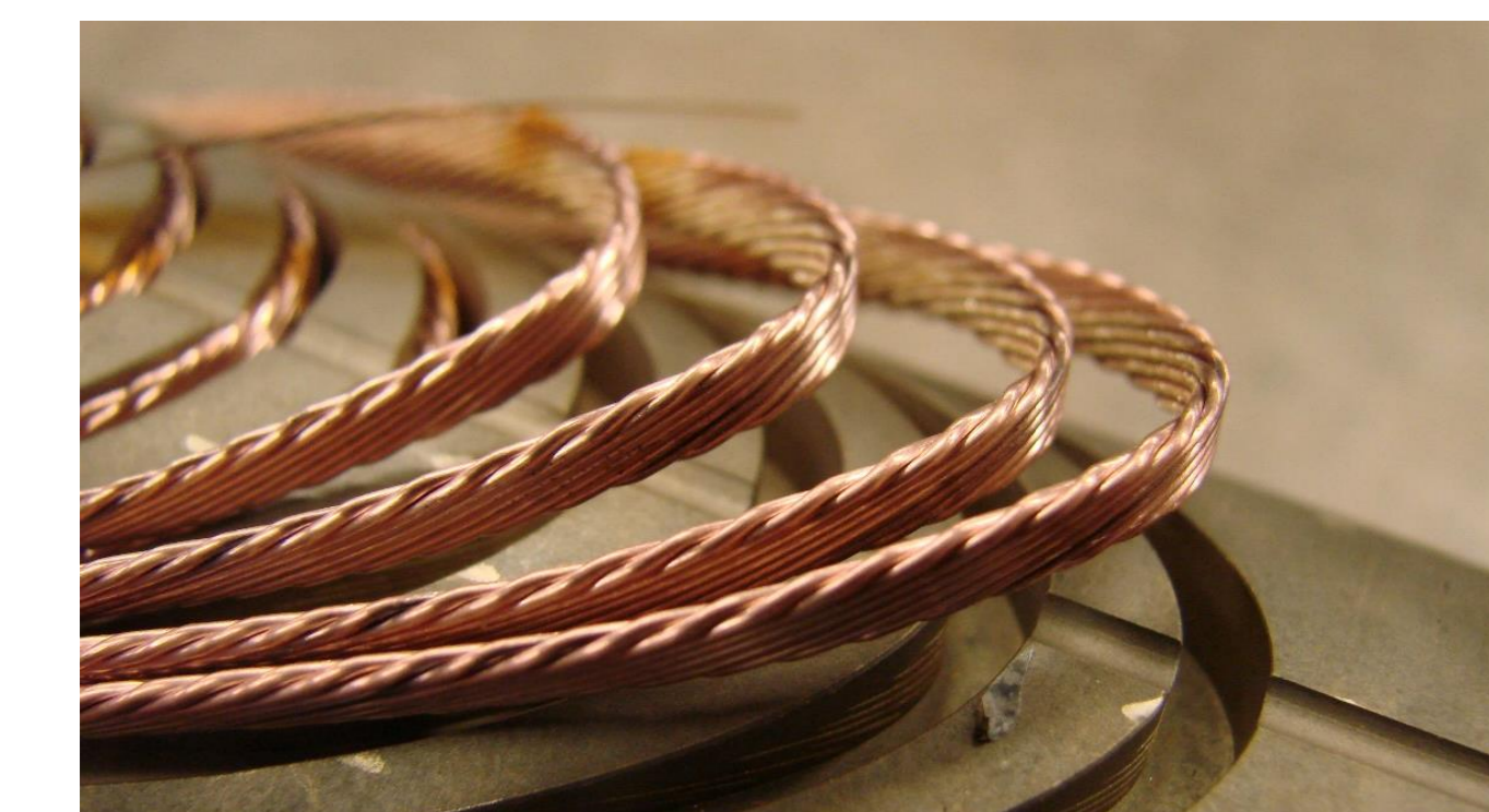
Next reaction test will incorporate mica or other standoff method to prevent sintering
