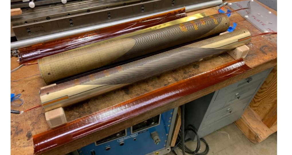
Assembly with inflatable shims
