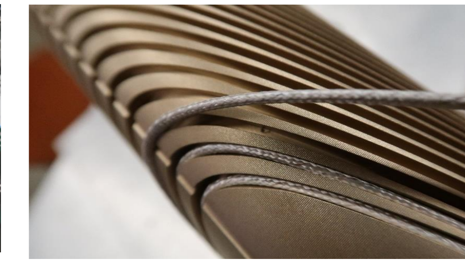
Layers wound with 11 strand cable of 0.6 mm RRP wire
