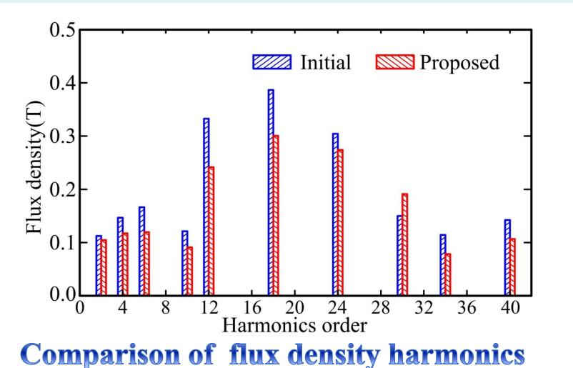
By optimizing  $\zeta$ , the air-gap flux density harmonics are reduced effectively, which indicates the rationality of this method.
