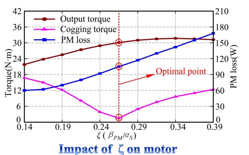
$\zeta$  is the key parameter of this method. The motor is improved taking PM loss, cogging torque and output torque into consideration
