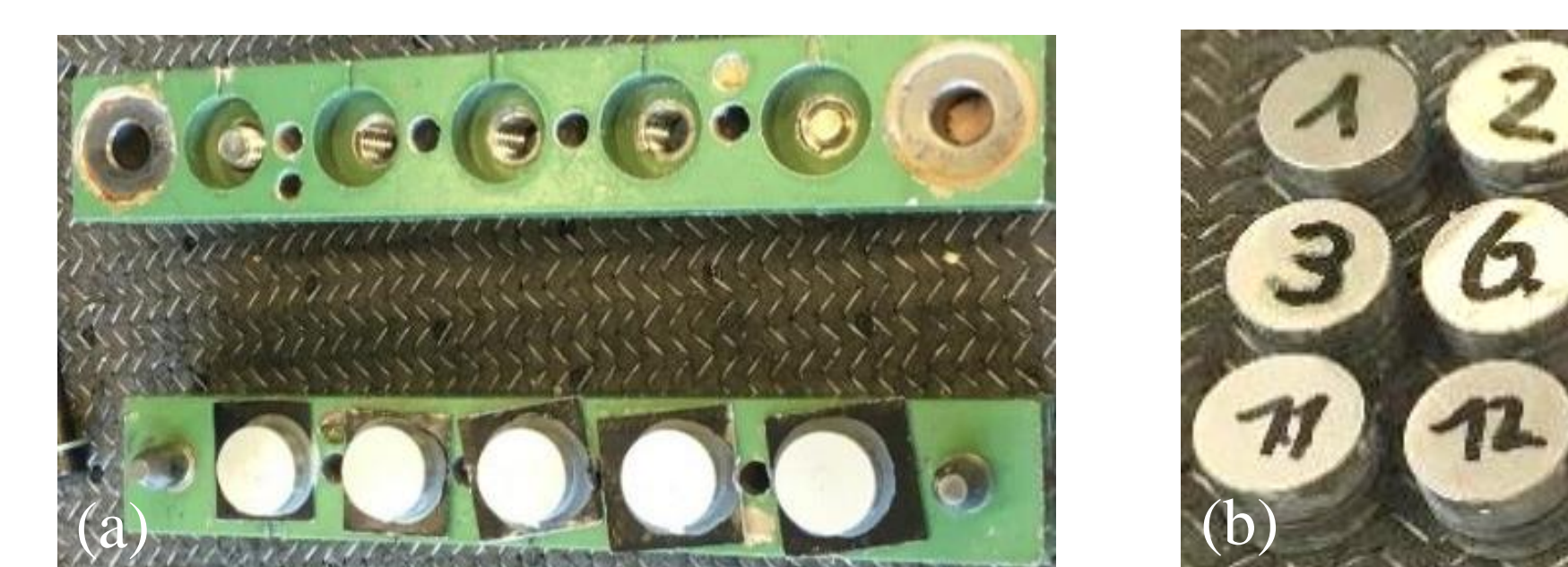
Tool for disk alignment and compression during glue curing (a) and paired cylindrical samples (b).
