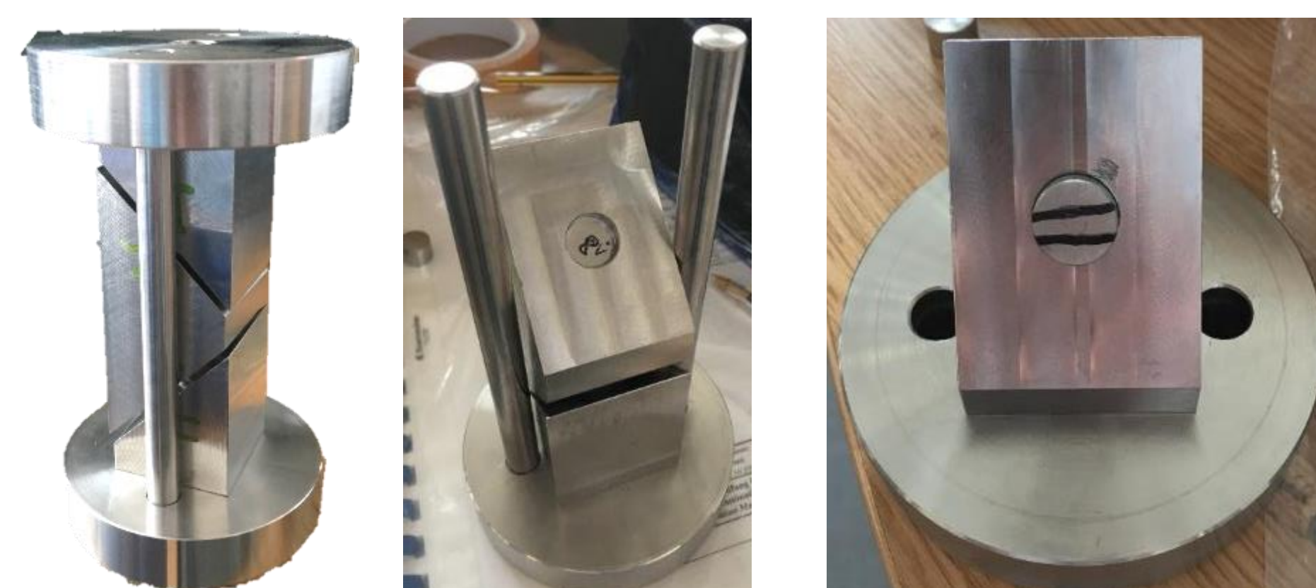
Stainless steel sample holder of the shear compressive test.
