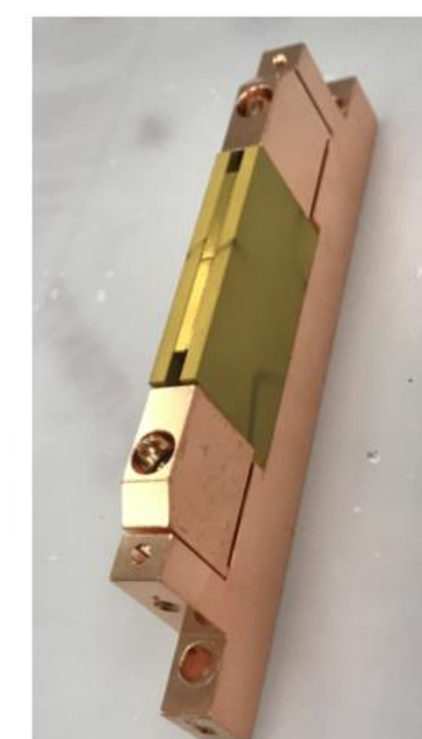
Magnetic module: half period unit, consisting of 2 magnet blocks and 1 pole piece
