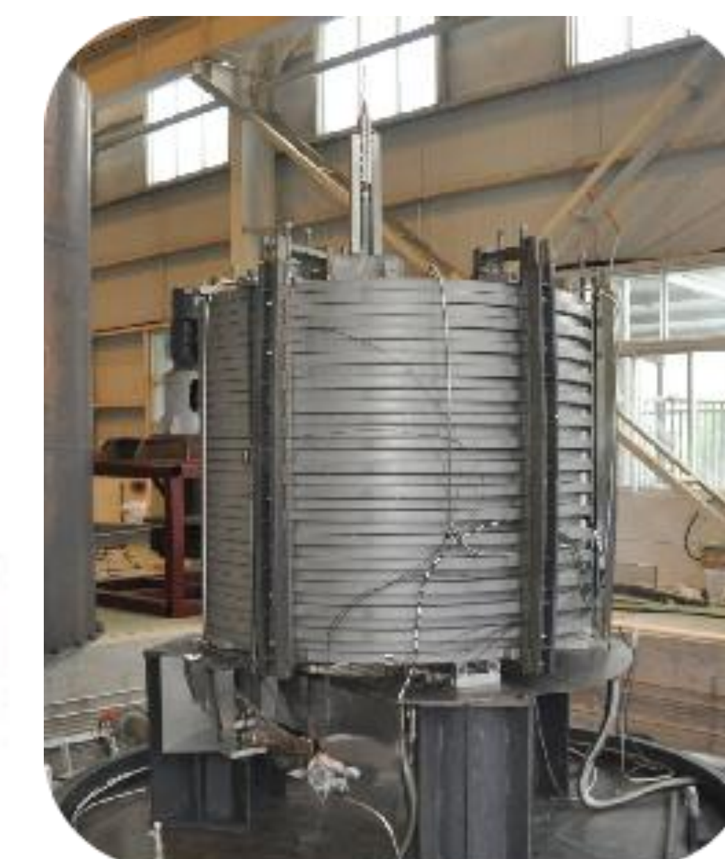
Figure 6 Nb 3 Sn inner coil assembled
