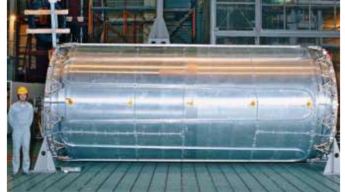
25 m 3 ATLAS Solenoid 8 kA @ 2 T, 40 MJ
