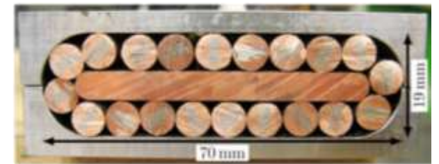
Swiss Plasma Center: Twisted Stacked Rectangular CICC
