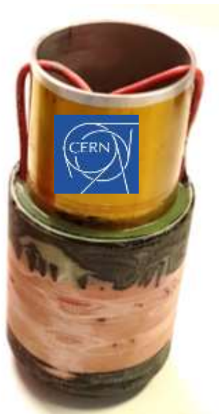
74mm dia, insert 2 layers, 2T in 15T
