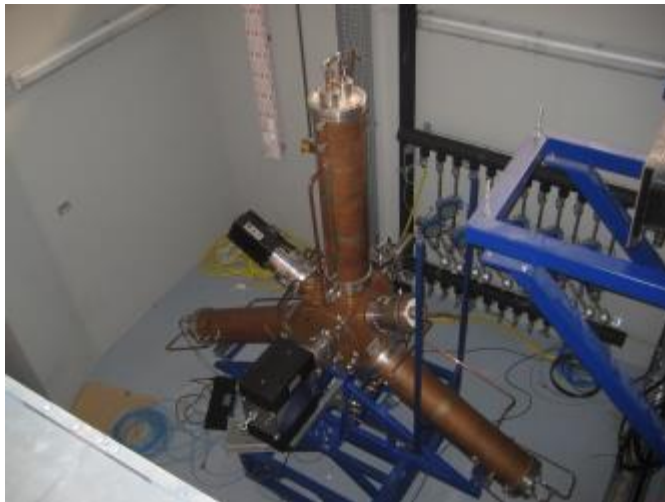
ALBA Cavity inside the Bunker
