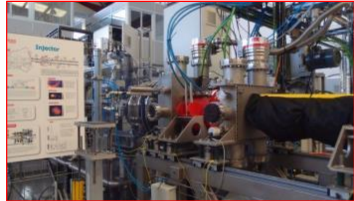
LEBT: Low Energy Beam Transport Focusing and beam diagnostics
