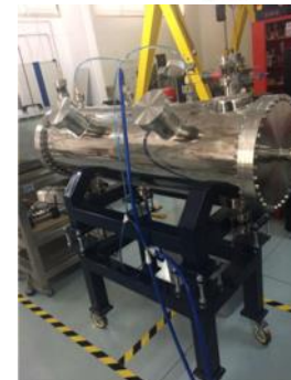
RFQ & IH prototypes being tested at CCTH – Huelva
