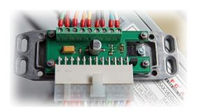
Device Under Test (APV25) with charge injection circuit NIM Pulser for Trigger TTL Pulser (synchronized) with Attenuator & Delay for charge injection
