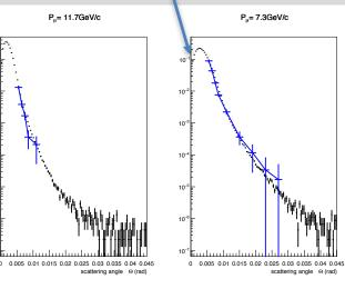
Description of multiple scattering and catastrophic energy loss, which may influence the muon shield performance, tested with existing data
