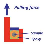
Wire impregnated with epoxy applied stress uniformly distributed
