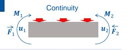
• Free to elongate and symmetric by translation:  $\mathbf{u}_1 - \mathbf{u}_2 = [q \quad 0 \quad 0]'$  with q such that forces and couples are null:
