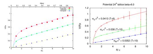
The static quark-antiquark potentials as functions of the quark-antiquark distance R: (from above to below) full  $V_{\rm full}(R)$ , restricted part  $V_{\rm rest}(R)$  and magnetic-monopole part  $V_{\rm mono}(R)$ . (Left) SU(2) at  $\beta=2.5$  on  $24^4$  lattice, [Kato, Kondo and Shibata, PRD $\mathbf{91}$ , 034506 (2015)] (Right) SU(3) at  $\beta=6.0$  on  $24^4$  lattice. [Kondo, Shibata, Shinohara & Kato, PRD $\mathbf{83}$ , 114016 (2011)]
