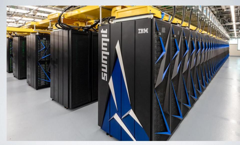
"Lattice Gauge Theory Machine" 200,000,000,000,000,000 Floats/sec 9,216 IBM POWER9 CPUs and 27648 NVIDIA GPUs Each GPU has 5120 Cores and total of 580,608,000,000,000 transistors
