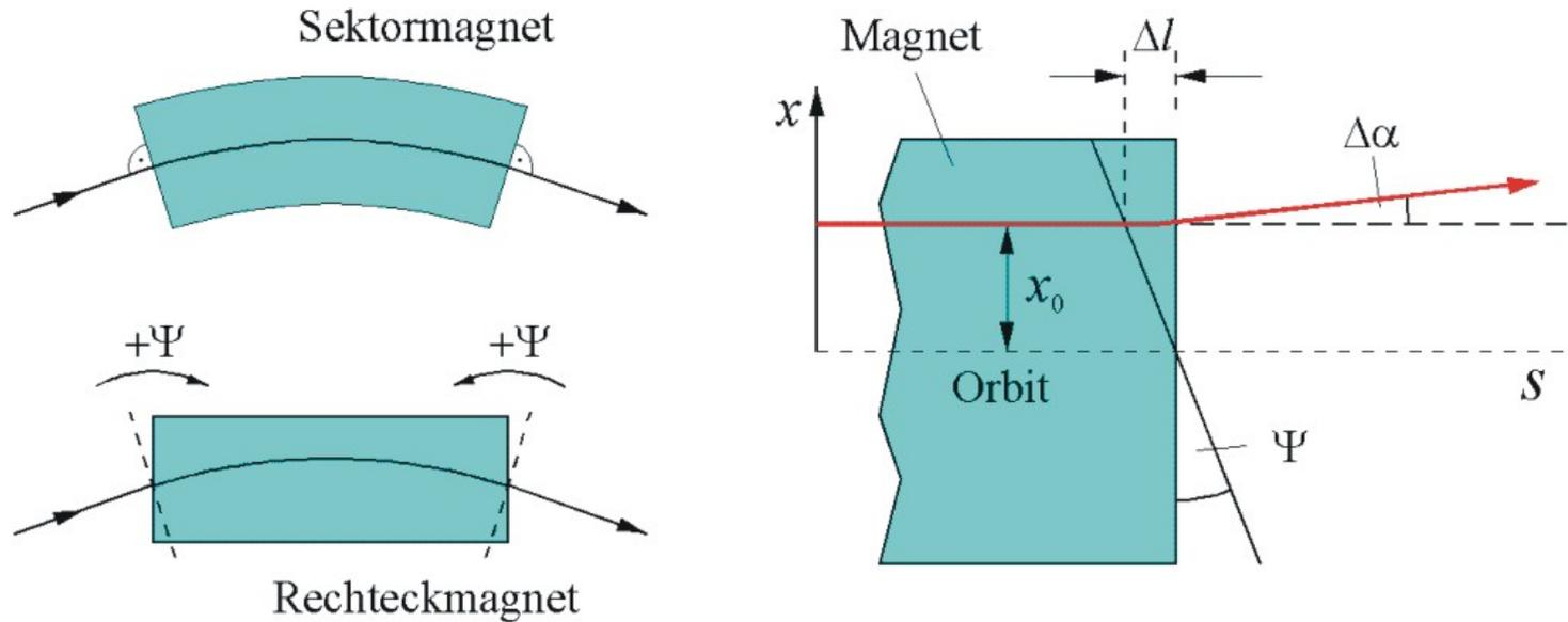
For a deflection angle  $\varphi$  we have an entrance and exit angle  $\psi = \varphi/2$ . The orbit of a particle traveling with a radial displacement  $x_0$  at the position of the magnet pole of a rectangular dipole is shorter than the reference orbit (with  $x_0 = 0$ ) by
