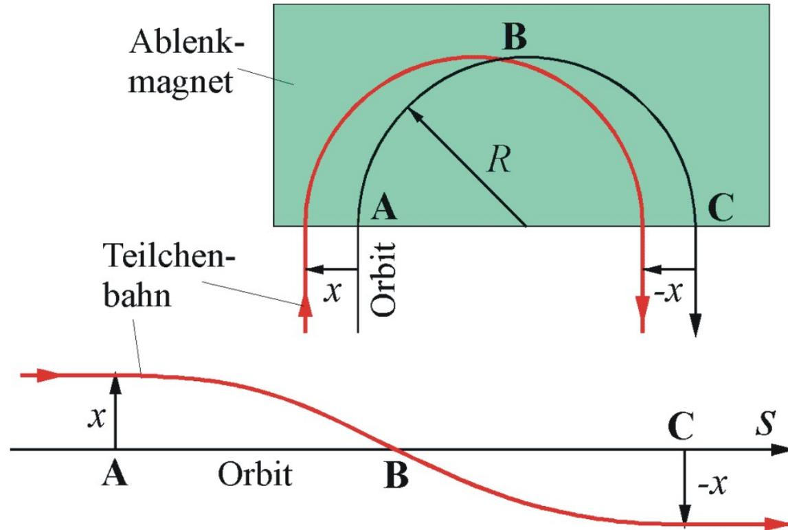
Due to technical constraints, particle accelerators often use rectangular magnets which have parallel end faces. Commonly these magnets are installed symmetrically about the intended particle trajectory:
