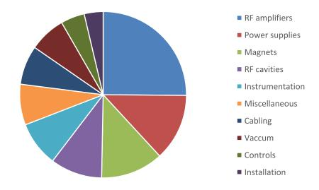
FIG. 7: The cost breakdown for PBS level 2.n.m as an illustration of detail level at this time. These technical domain sums are the results of costing 80 individual sub-components for this PBS level.
