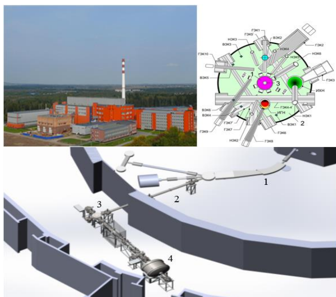
Fig. 4.3. Collage of the reactor PIK properties [1, 2] with basic characteristics: power: 100 MW; thermal neutron flux: 5 \times 10^{15} n/cm 2 sec. In the bottom of figure - arrangement of the setup PITRAP (4) is shown. It will use the horizontal channel ГЭК 5 and the electromagnetic mass separator (1) followed by ion channel (2) and bending dipole magnet (3).
