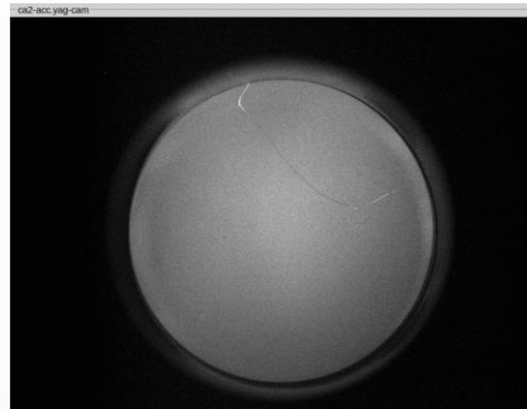
CeC: 8/18 – Crack (ca2-acc.yag)
