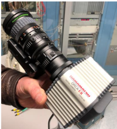
Hamamatsu ORCA-ER deep cooled CCD camera with motorized lens and microscopy software
