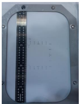
AGS-to-RHIC PM screen with ruler for resolution measurements
