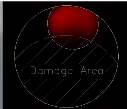
Part of YAG still sensitive to beam – dead lower center
