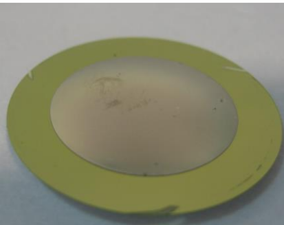
Damaged YAG removed from aluminum holder
