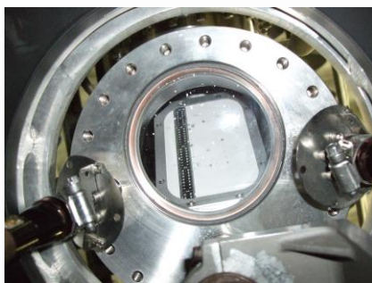
AGS-to-RHIC PM screen with ruler for resolution measurements
