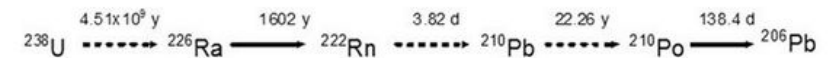
Figure 2: ^{238}\text{U} decay series, showing the principal radionuclides concerned with the production of ^{210}\text{Pb} and their radioactive half-lives.
