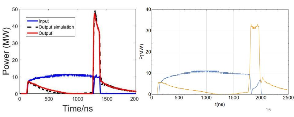
High power tests of the compressor
