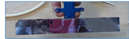
ITS Outer Barrel HIC. 14 pixel sensor chips are mounted on a flexible printed circuit
