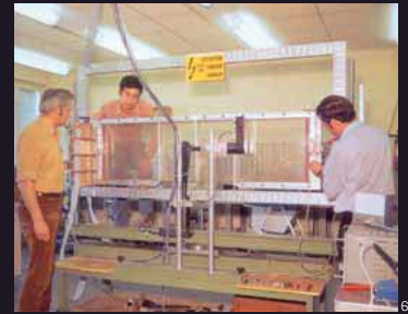
5, 6. For decades, studying particle trajectory at CERN relied on examining by hand millions of photographs from bubble chambers like the Big European Bubble Chamber (pictured here). In 1968, Nobel prizewinner Georges Charpak (below, left) brings particle detection into the electronic age with his "Multiwire Proportional Chamber" (MWPC). Using transistor amplifiers and linked to a computer, his invention allows for a 1000-fold increase in detection rate.
