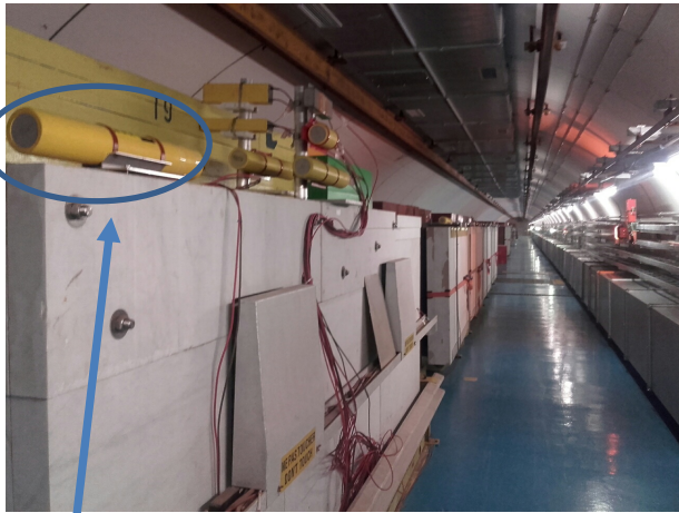
TT66.BLM.660518LOSS_EXTR1 next to the last BTV on the beamline (just before the beam exit window) TT66.BLM.660523LOSS_EXTR1 next to table B (where your experiment is installed) TT66.BLM.660526LOSS_EXTR1 next to table C (most downstream table)
