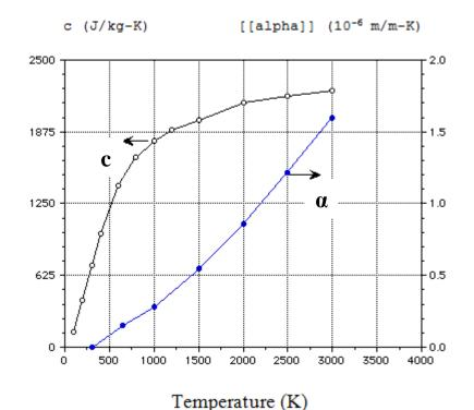
**Specific heat** and coefficient of thermal expansion of pyrolytic graphite.
