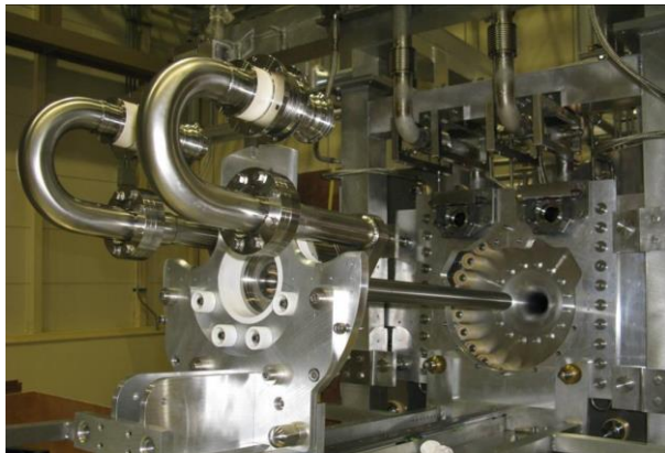
T2K helium-cooled carbon target (C. Densham)
