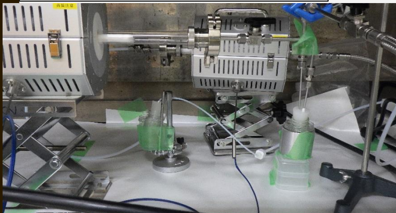
Two tube furnace and 3\text{H} traps, which can distinguish HT with HTO.
