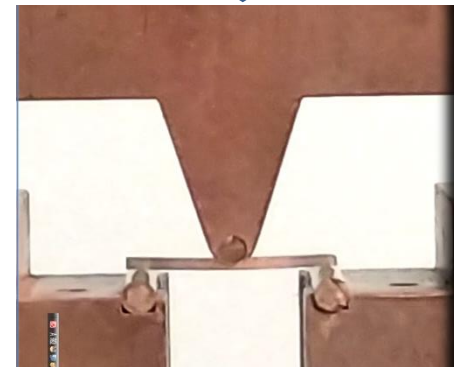
Specimen deflection during 3PB testing 40
