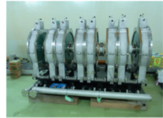
- New 2nd harmonic cavity with 4 accelerating gaps
