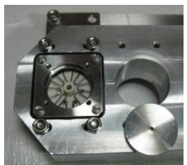
Temp. Calib. Heater+Be plate, TC
