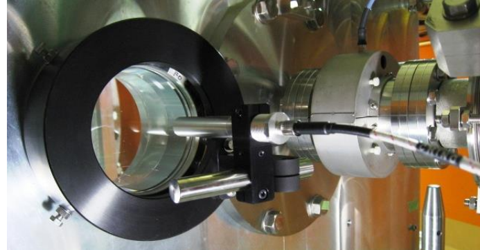
Sapphire view port & Lenz unit mounted on the Target chamber
