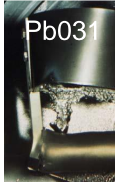
Welding rupture in window of molten lead targets (not an issue observed with solid targets at >2000C)
