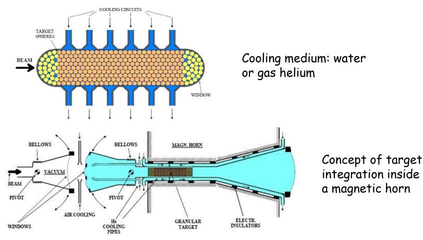
P. Sievers's proposal of a granular target at CERN (2001)
