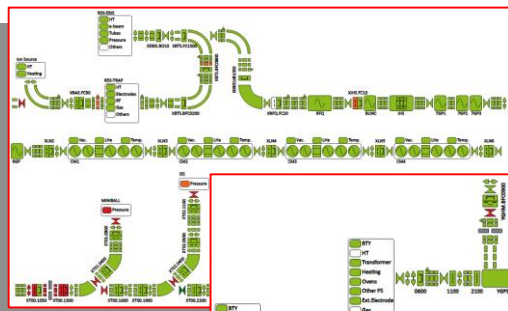
GUI of the Fast Beam Investigation (FBI) software (E. Fadakis, E. Matli, BE-OP-ISO)
