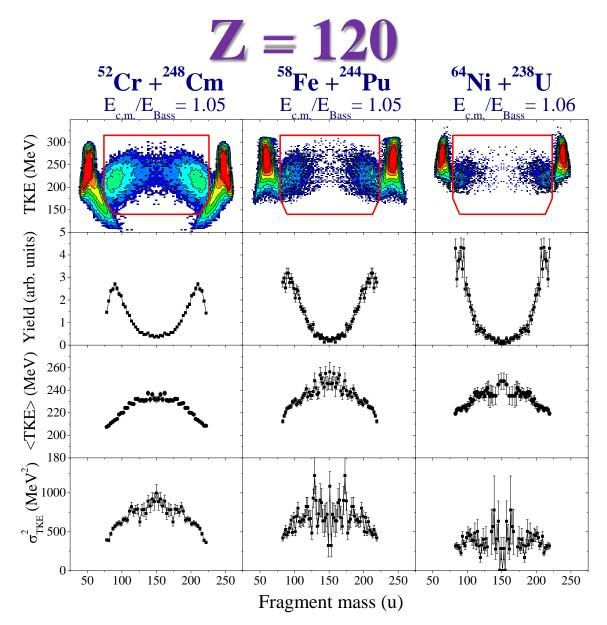
The mass and energy distributions of binary fragments formed in the reactions  ${}^{52}Cr + {}^{248}Cm$ ,  ${}^{58}Fe + {}^{244}Pu$ , and  ${}^{64}Ni + {}^{238}U$ , leading to the formation of composite systems with Z = 120 at energies above the Bass barrier. From top to bottom: the M-TKE matrices of binary reaction products; the mass distributions; the average total kinetic energy and its variance as a function of mass of fissionlike fragments inside the contour line on M-TKE matrices
