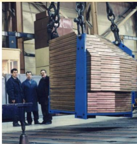
Manufacturing of 2 hadronic wedge calorimeters for CMS Detector (Felguera Construcciones Mecánicas S. A. (Barros, Spain))
